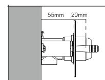
Ensure the valve is set back from the finished front face of the wall by the correct depth of min 55mm max 75mm depending on which tap (Allow for tiles, adhesive, etc).
