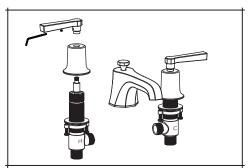
Once the body and handles are in place, make sure to tighten the fixings on the valves and body to secure them to the basin.
